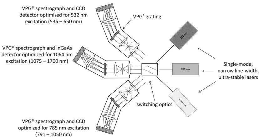
A simple design of three-excitation (532, 785, and 1064 nm) laser Raman system which can be a stand alone spectrometer or integrated into Raman microscopes. In this design, as each spectrograph/detector is only used for its unique wavelength band (no sharing), the system can maintain high response for an extended range of wavelengths (e.g., from UV to NIR).
