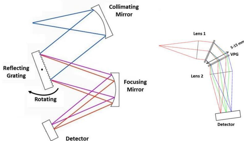
**Left**, schematic diagram of a traditional spectrograph based on a reflecting grating. Adapted from James B. Kaler, Stars and their Spectra: An Introduction to the Spectral Sequence Cambridge University Press (March 28, 1997). **Right**, VPG design allows high compactness and no moving parts in the system.
