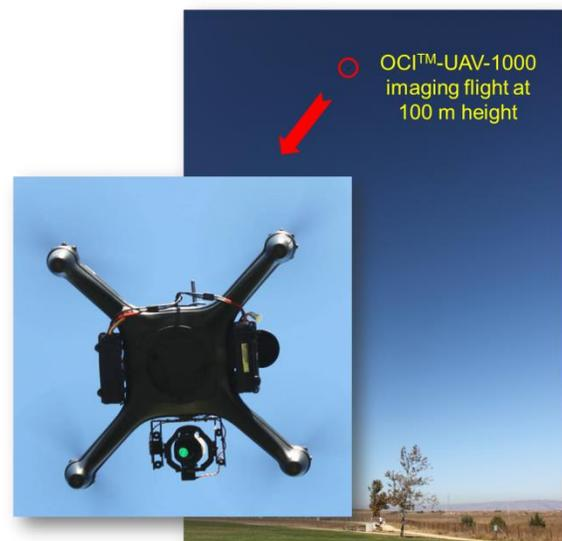
**Figure 1.** BaySpec's OCI™ hyperspectral imagers are ultra-compact and light weight (0.3 kg total), designed specifically for use on sUAVs. Shown in the photo is the system in aerial hyperspectral imaging mission.
