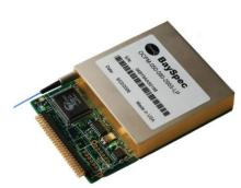
BaySpec's OCPM Series Optical Channel Performance Monitor is an embedded, integrated spectrum analyzer delivering precise measurement and powerful processing capabilities for dense wavelength division multiplexing (DWDM) applications.
