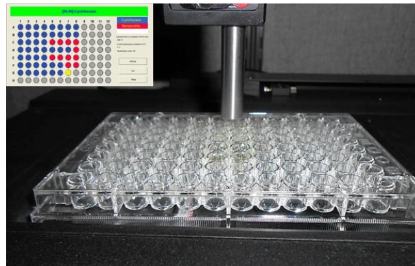
Figure 6: 96-well micro-plate sampling accessory for automatic Raman acquisition. Inset: software interface during an automated measurement with Identification Mode on.
