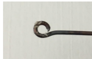
Figure 3. Close-up of wheat powder on the inoculation loop of the Sample Probe
