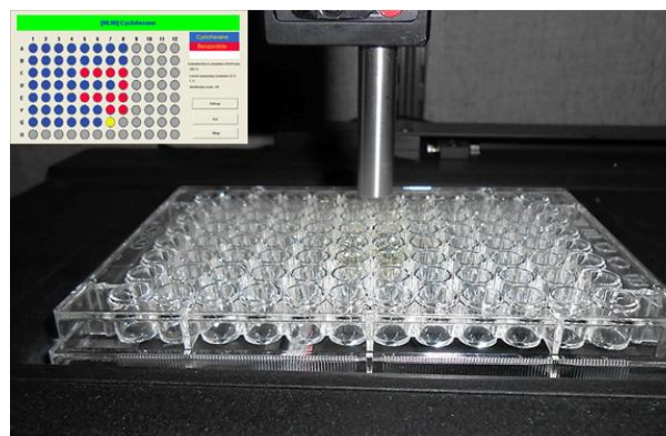
Figure 5: 96-well micro-plate sampling accessory for automatic Raman acquisition. Inset: software interface during an automated measurement with Identification Mode on.
