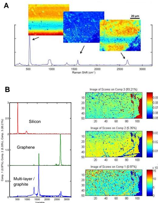
**Figure 2.** (A) Direct Raman chemical imaging of a graphene sample on silicon substrate. Raman images are reconstructed by silicon's 520  $\text{cm}^{-1}$  peak, graphene's G band, and G' band. (B) Further chemometric analysis (Multivariate Curve Resolution, MCR) are performed using Solo+MIA (optional package included in *Nomadic*'s Spec20/20 software suite). Components (silicon, graphene and graphite) distribution can be quantitatively revealed.
