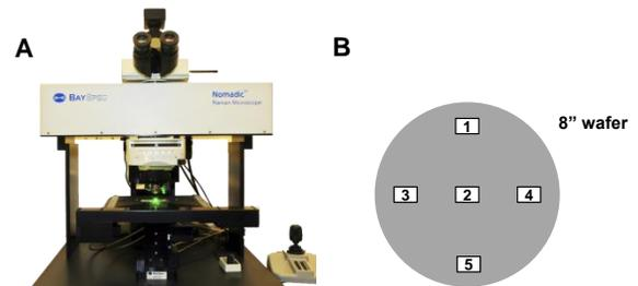
**Figure 1.** (A) *Nomadic*<sup>TM</sup>-532 large-format Raman microscope. (B) Regional mapping function can automatically scan multiple pre-defined sites on a large sample (e.g., 5 sites on an 8" wafer).
