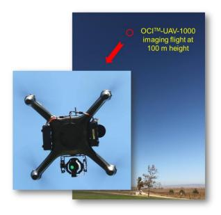
**Figure 1.** BaySpec's OCI<sup>TM</sup> hyperspectral imagers are ultracompact and light weight (0.3 kg total), designed specifically for use on sUAVs. Shown in the photo is the system in aerial hyperspectral imaging mission.
