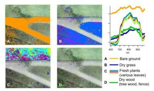
Figure 3. A "material map" generated automatically from hyperspectral data cube based on each material's spectral characteristics.
