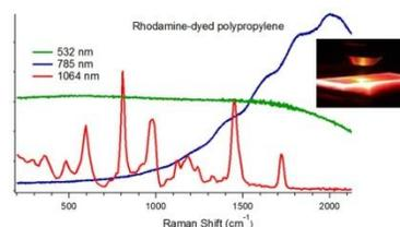
**Figure 1.** In real-world, most materials are colored. 1064 nm is perfect for Raman spectroscopy of colored materials (shown here is a piece of rhodamine-dyed plastic slide).
