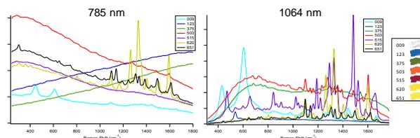
**Figure 2.** Most paint and ink, or even just some white paper, are highly fluorescent under visible laser illumination. Only 1064-nm excitation produces high-quality, signature-rich Raman spectra for these samples. Shown here are 785 and 1064-nm Raman spectra of some oil paints.
