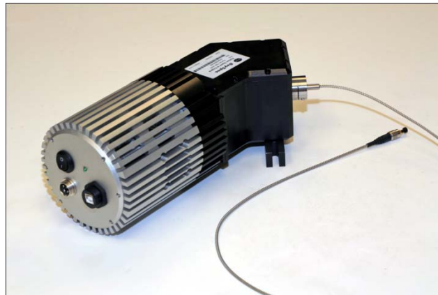
Figure 8: Nunavut TM Deep Cooled Detector coupled to a typical BaySpec NIR spectrograph
